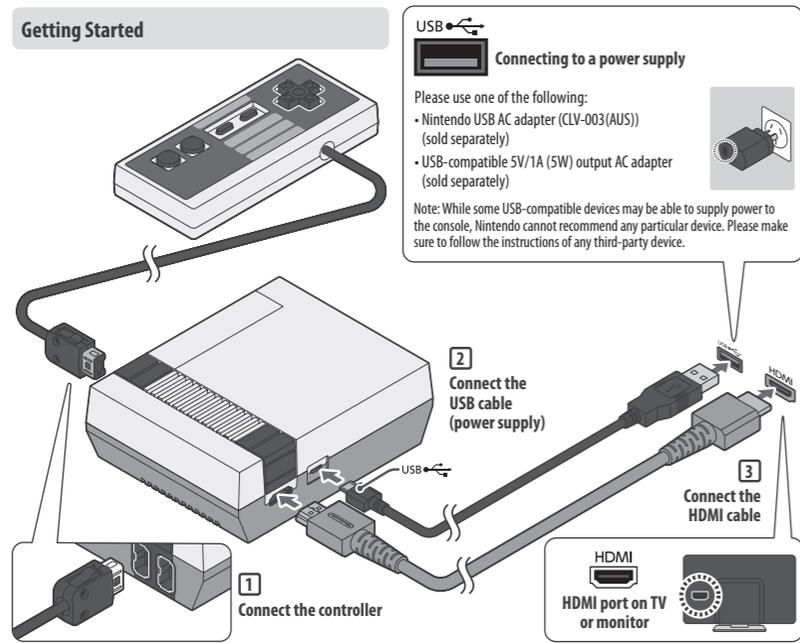
**WARNING** Make sure the connectors on the cables are oriented correctly and then insert them straight into the correct ports.
