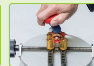
Checks whether parts easily break when twisted and, if so, whether they break off safely
